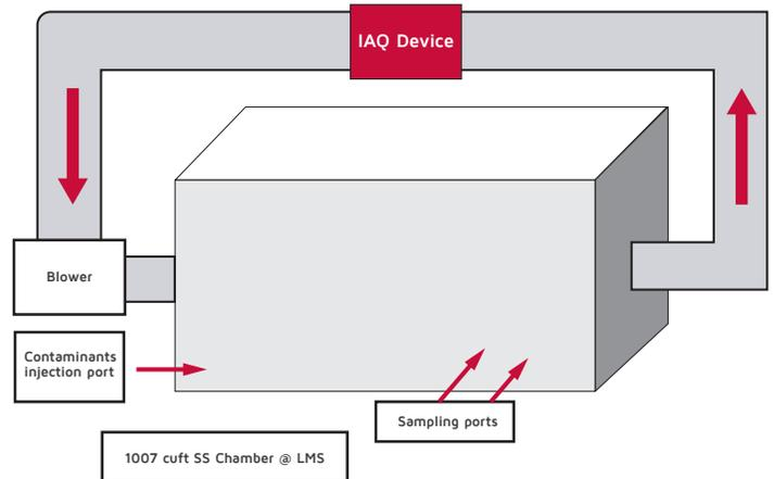
**FIG. 3** Rendering of the Multi-pass system showing the duct arrangement, injection port, air samplers
