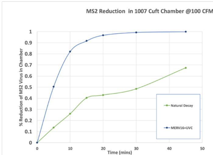
**FIG. 5** Percent reduction vs time MERV 16 + UVC @ 100 CFM
