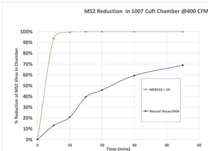
FIG 6. Percent reduction vs time MERV 16 + UVC @ 400 CFM
