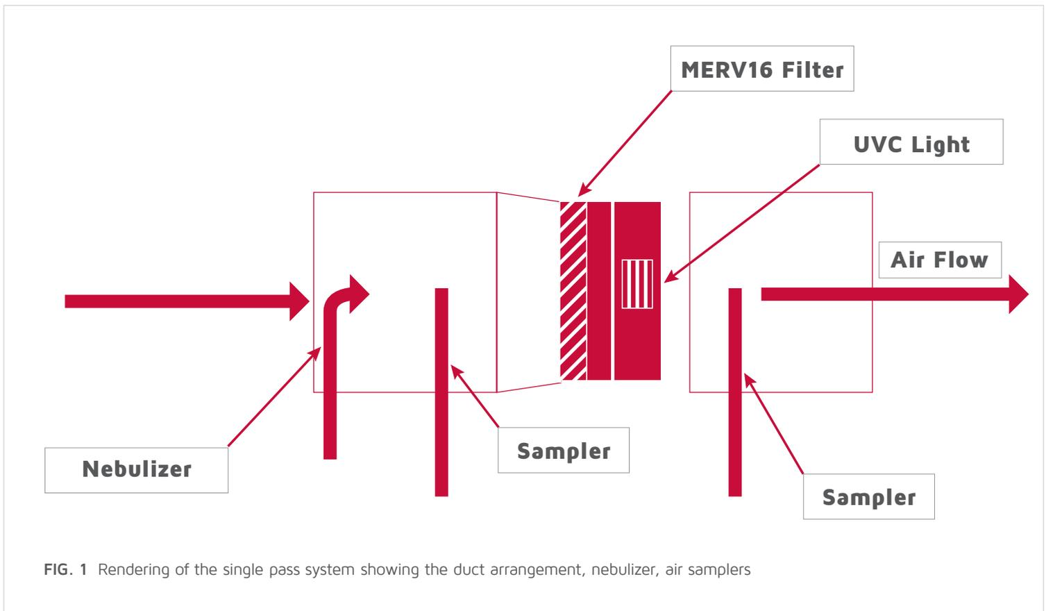
**FIG. 1** Rendering of the single pass system showing the duct arrangement, nebulizer, air samplers
